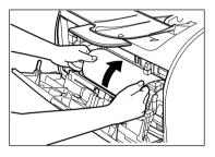
5 Roll the leading end of the paper outwards so that the printed surface is on the inside of the roll, then gently pull the rolled up paper out of the machine.
